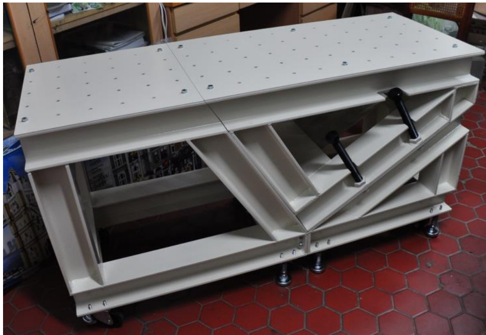
Figure 2.31. The first shear banding table available in the world
