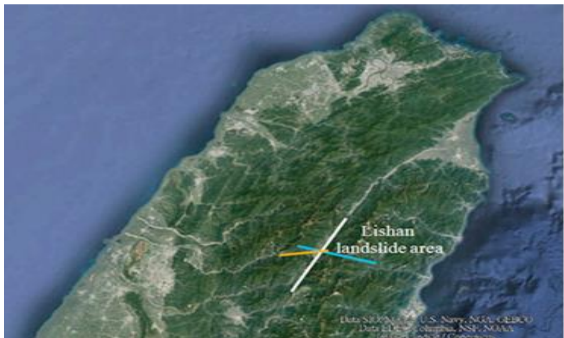
Figure 5.3. Lishan landslide area is the intersection zone of three shear bandings (background picture is from Google Earth, 2017)
