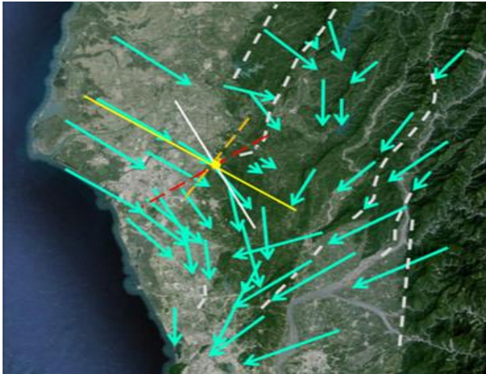
Figure 7.8. Shear bands identified from the distribution of displacement velocity vectors (background figure and vectors taken from Google Earth (2017) and GPS LAB (2017), respectively).
