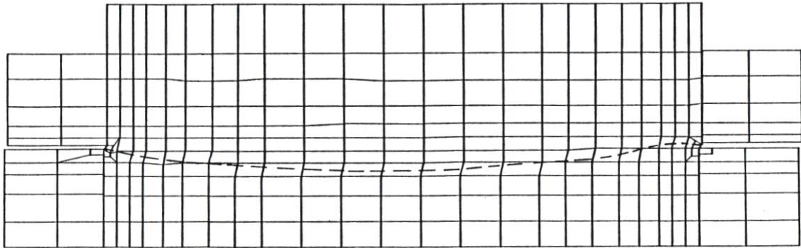
Figure 1.92. Numerical simulation of direct shear test (Size of gape = 0.025 inch, doubled normal stress and shear strength of the interface elements)
