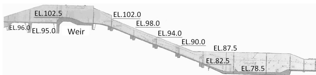
Figure 3.59 Sectional view for the spillway of Renyitan Reservoir (ZTE Engineering Consultants Co. Ltd., 2008)
