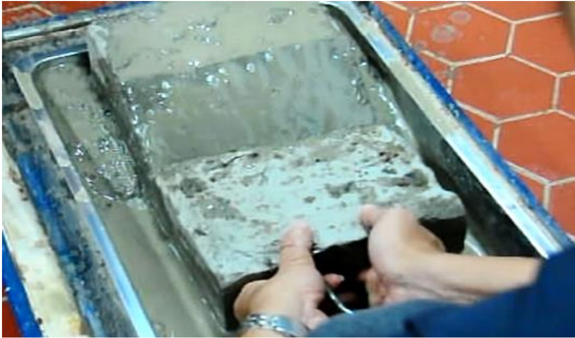
(b) After ground water flow upward with sediment entrainment
