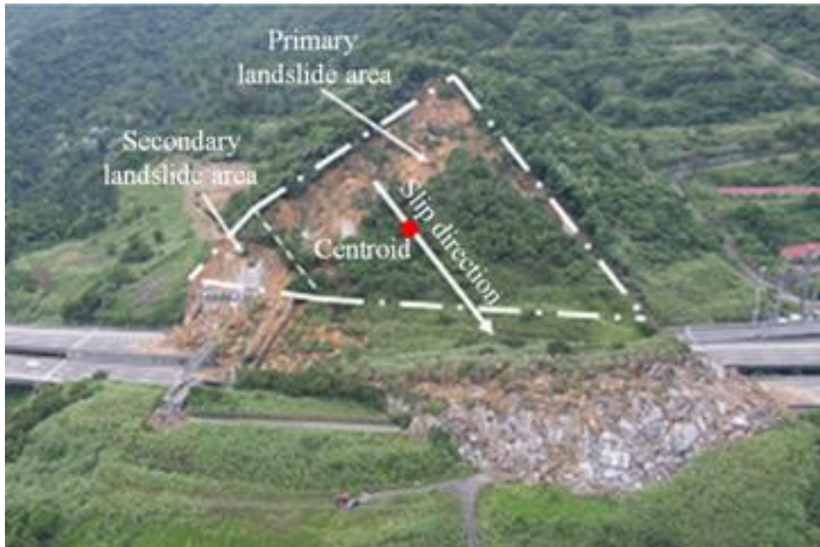
Figure 6.6. The slip areas adopted by the authors (background image from Taiwan Geotechnical Society, 2011).
