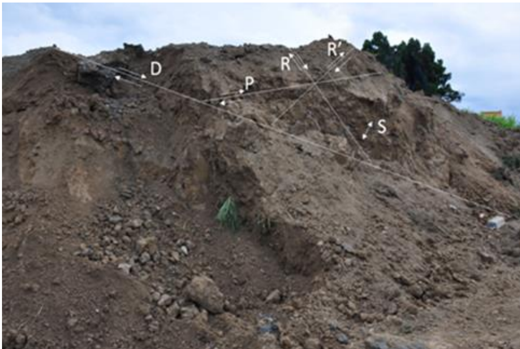
(c) In-situ shear bands caused by the 2016 Meinong Earthquake.
