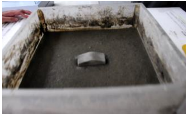
(b) Only punching shear failure produced after vibrating
